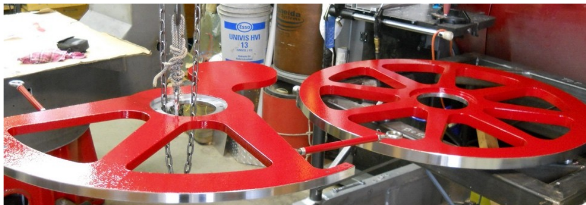
Figure 7. The notorious new altitude drive sector (left) and azimuth drive wheel (right) after painting in Roman's shop. Photo by Roman Unyk.
