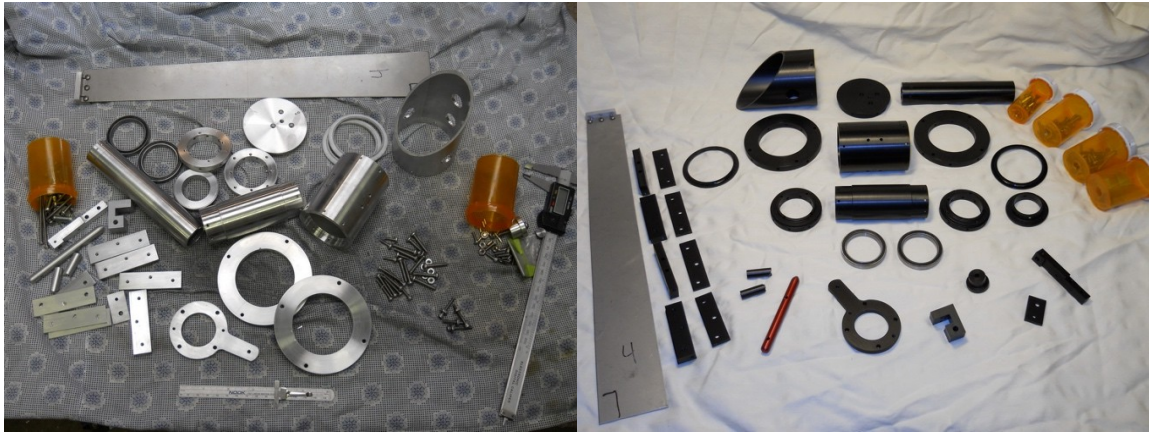
Figure 6. The components of the tertiary mirror holder, machined by Roman, before and after anodizing. Photo by Roman Unyk.
